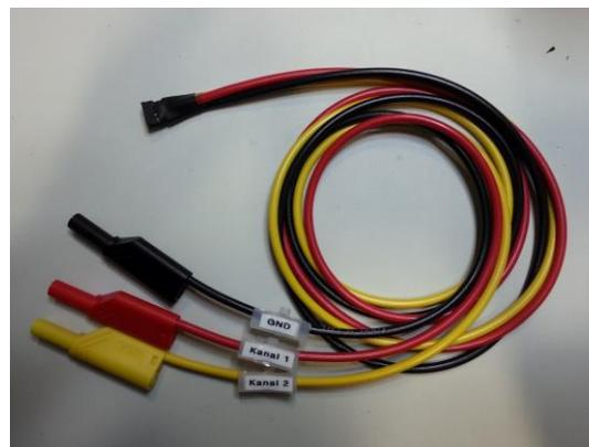
Figure 2 – Measuring adapter
