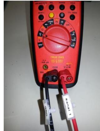
Figure 9 – Connection for channel 1
