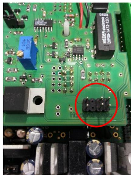
Figure 6 – Connection on the circuit board for the measuring adapter
