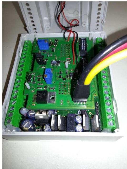
Figure 8 – Module with connected adapter
