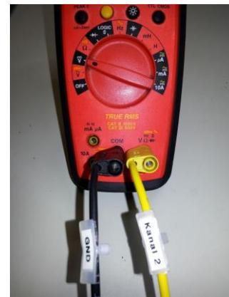
Figure 10 – Connection for channel 2
