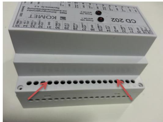
Figure 4 – Position of the clips
